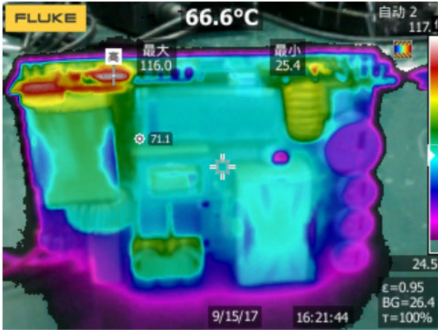
Figure 44. 90 Vac & 48 V 5 A, Front Side
