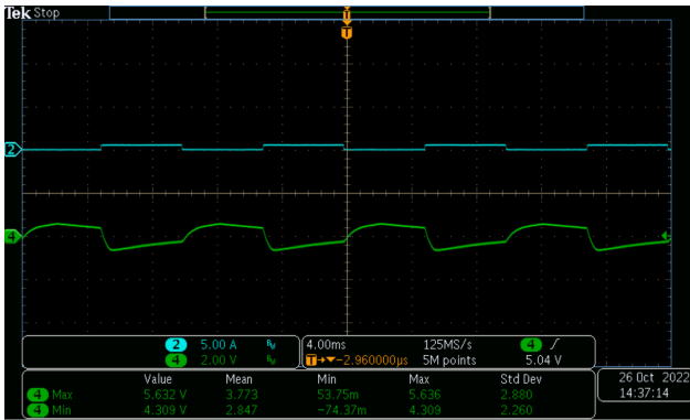
Figure 38. 5 V & 0 A to 0.5 A, 10 ms Cycle, 0.25 A/ \mu s (ch2-lo, ch4-Vo)
