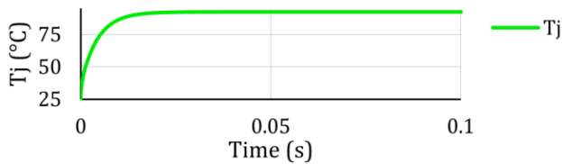
Figure 39. Temperature with Continuous Drain Current @ Stable T_A
