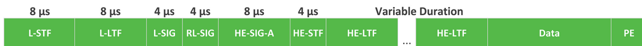
Figure 1. Structure of an 802.11ax Packets Showing HE-LTF Fields Used for CSI Measurement
