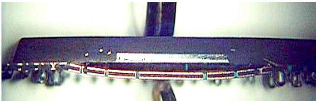
Figure 102. BGA Cross Section Exhibiting Moisture Damage (Popcorning)
