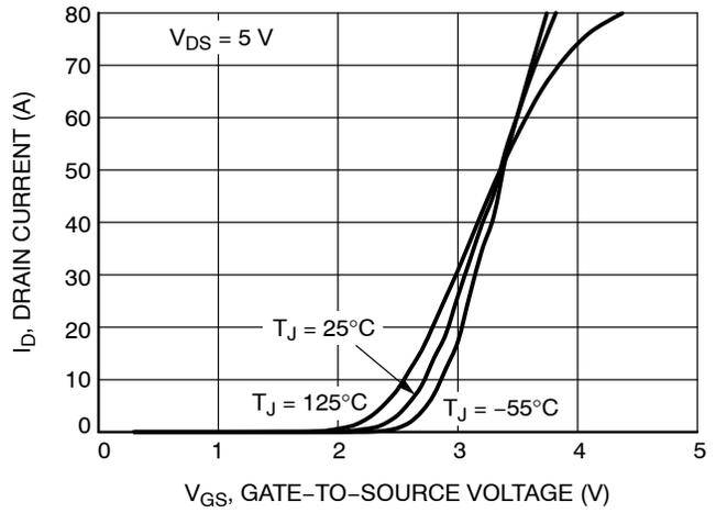
Figure 2. Transfer Characteristics
