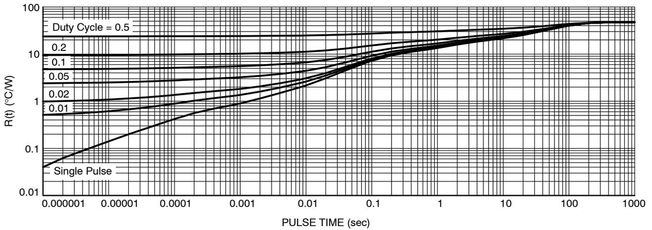
Figure 13. Thermal Characteristics
