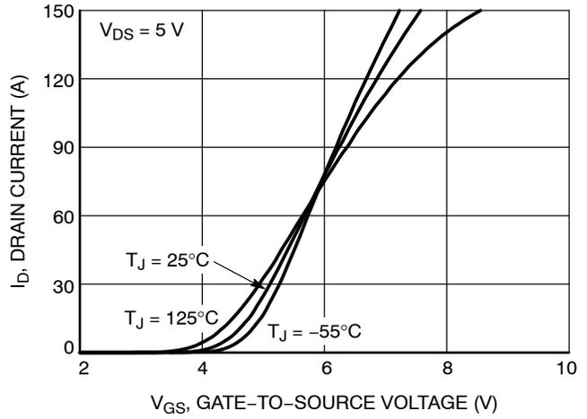
Figure 2. Transfer Characteristics
