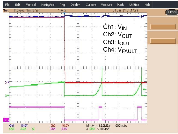
Figure 19. I_{TH} Overcurrent Event on Auto-retry Device
