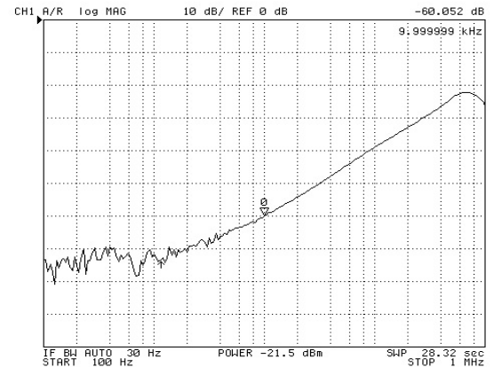
Figure 15. LDO5 PSRR vs. Frequency, 150 mA Load
