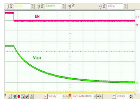
Figure 27. Shutdown, No Load, Output Discharge Enabled
