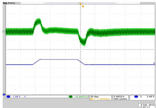
Figure 14. Line Transient, 200 mA Load, 10 μs Step
