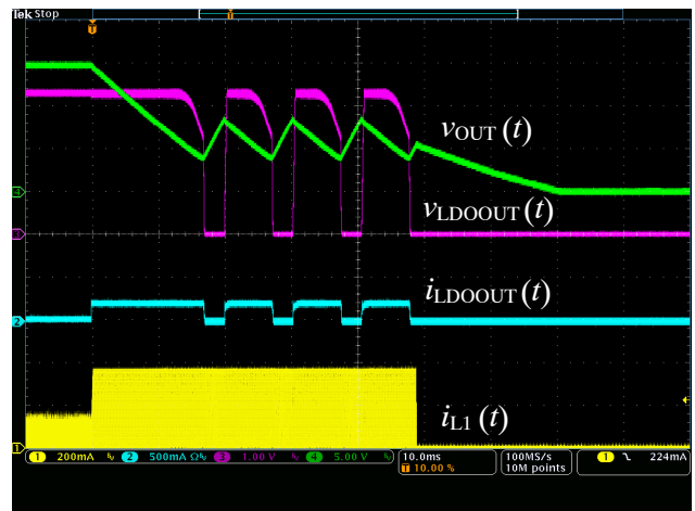
Figure 34. LDO Over-current Protection – Over-loaded LDO Rail, I_{OUT} = 30\text{mA} , I_{LDOOUT} = 30\text{ to }200\text{mA} , V_{IN} = 230\text{V}
