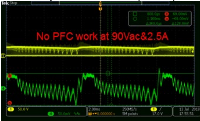
20V2.5A output without PFC work(CH4: Vo)
