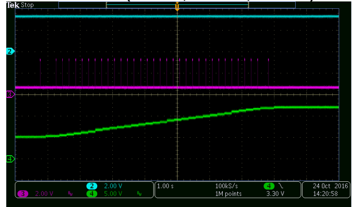
QC3.0 CNT Mode (CH2: D-, CH3: D+, CH4: Vo)
