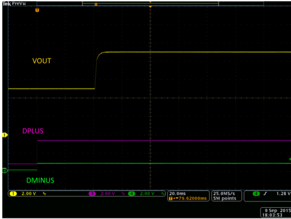
Figure 14. Transition from 5.0 V to 9.0 V
