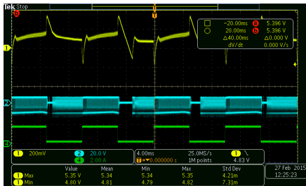
Figure 13. Test Conditions: 0.2–1.8 A, 250 mA/ \mu s, 10 ms Cycle, 115 Vac
