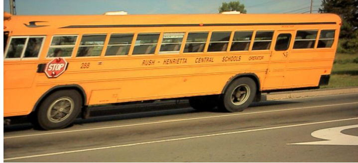
Figure 1. This Image of a Bus was taken using a CMOS Imager in Rolling Shutter Mode
