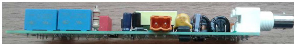
Figure 4. EVB Side Picture: Board Height is 15 mm
