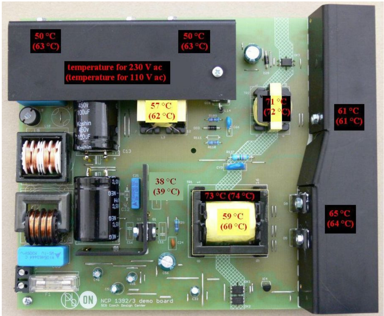
Figure 51. Photo of the Demoboard with Temperatures Measured for 230 Vac and 110 Vac in Bracket (Ambient Temperature 26°C, Full Load, Vertical Position)
