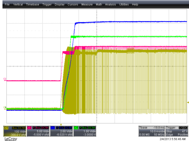
Figure 10. Startup Time = 9 ms, 300 V AC , No-Load Condition (CH1: V DS (100 V/div), CH2: V CC (5 V/div), CH3: 12 V OUT (2 V/div), CH4: 5 V OUT (1 V/div), Time: 10 ms/div)
