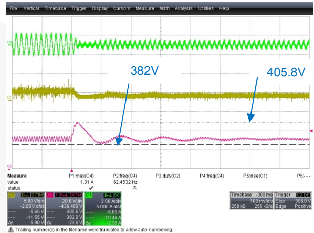
Figure 43. V IN = 235 V AC , P O = 160 W → 30 W
