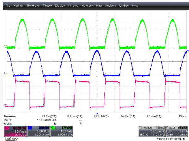
Figure 48. V_{PFC} = 400 V, P_O = 100 W; CH2: V_{D201} (100 V / div), CH3: I_{D201} (1 A / div), CH4: I_{D202} (1 A / div)
