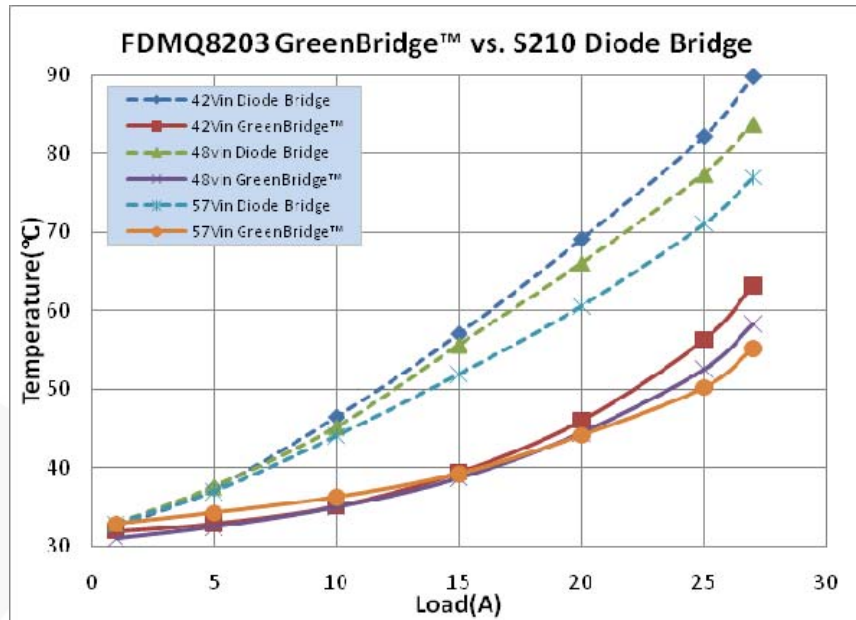
Figure 7. Thermal Performance Comparison: GreenBridge™ vs. Diode Bridge at V_{OUT}=3.3 , f_{SW}= 300 kHz, Soaking=3 Minutes, T_A=25^\circ\text{C}
