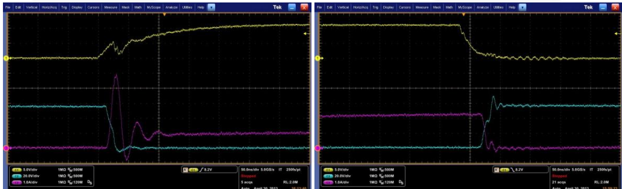
Turn-On Waveforms, Time (50 ns/div)
