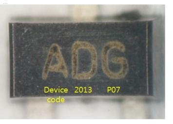
Description of Change (To) : Laser Marking layout based on Weekly code.
