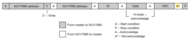
Figure 6. Format of I2C Write Access Frames
