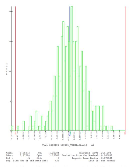
Current Cpk (spec limits) is 1,44. New cpk (new spec limits) with shifted spec window is 1,93.
