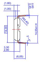
NOTES: UNLESS OTHERWISE SPECIFIED A) THIS PACKAGE DOES NOT COMPLY TO ANY CURRENT PACKAGING STANDARD B) ALL DIMENSIONS ARE IN MILLIMETERS C) DIMENSIONS ARE EXCLUSIVE OF BURRS, MOLD FLASH, AND TIE BAR EXTRUSIONS D) ( ) IS REFERENCE
