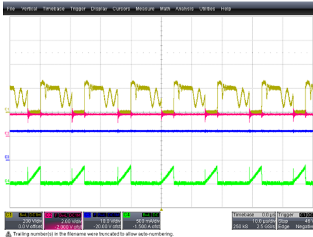
Figure 11. Full-Load Condition, 90V AC , (CH1: V DS (200V/div), CH2: V FB (2V/div), CH3: V CC (10V/div), CH4: I DS (500mA/div), Time: 10µs/div
