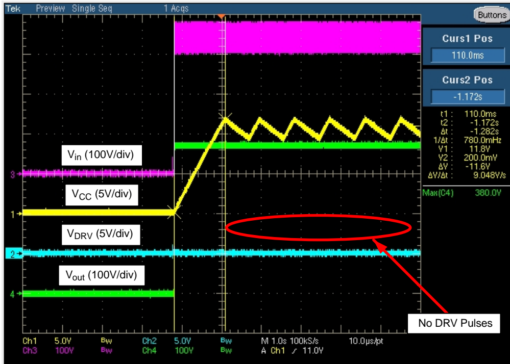
Figure 31. Startup with Jumper Removed ( V_{in} = 265 \text{ Vac } 50 \text{ Hz} , I_{out} = 0 \text{ mA} )
