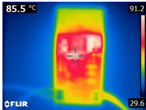
Figure 9. Thermal Image at 15.0 A Load
