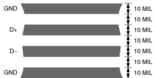
Figure 17. Arrangement of Signal Tracks
