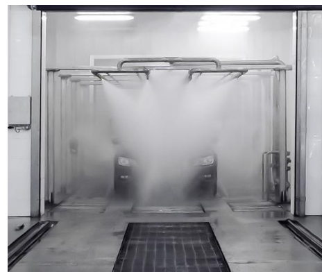
Figure 1. Automakers Turn Up the Pressure to Find Leaks with Water Jets in the 2,000 psi Range
