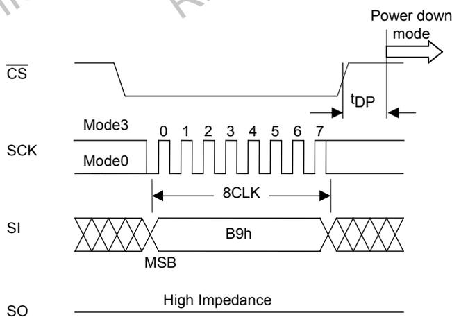
Figure 11. Exiting from Power-down
