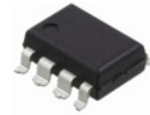
PDIP-7 MISSING PIN GW CASE 707AA
