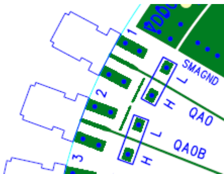
Figure 4. LVPECL Output Configuration
