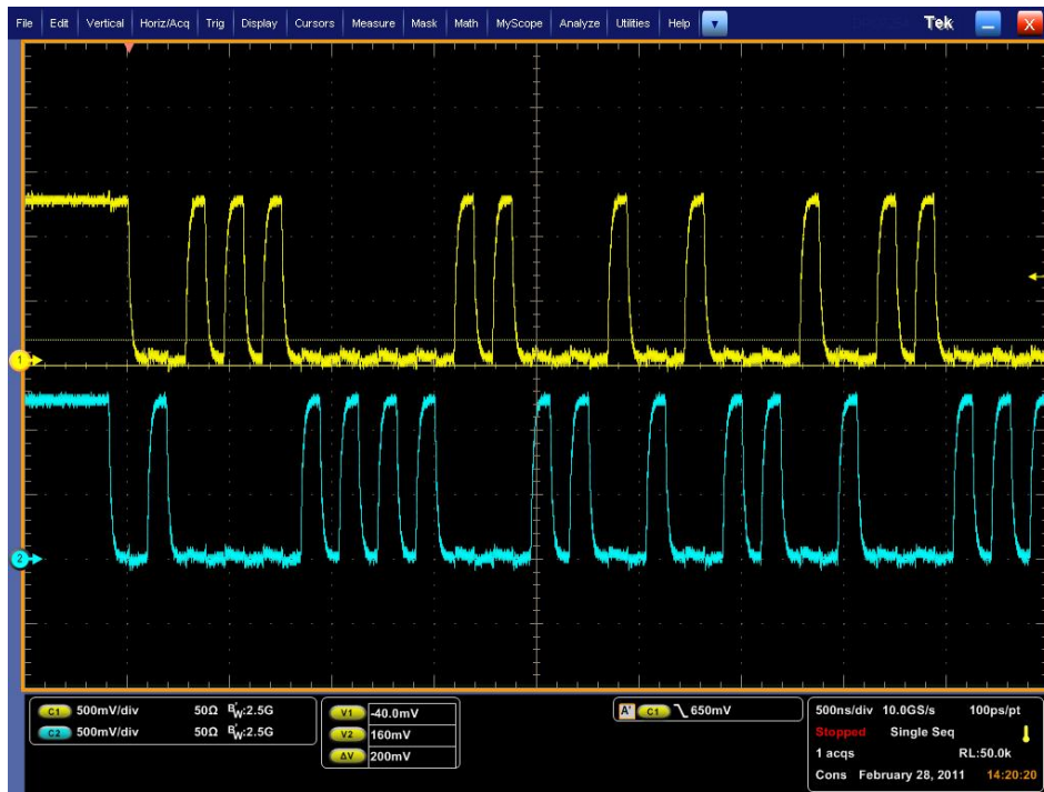
Figure 5. EMI4172 MIPI D-PHY LP Mode Measured Results
