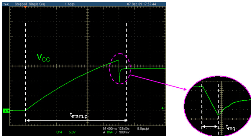
Figure 12. V_{\text{CC}} Waveform during Startup
