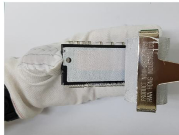
Thermal compound being applied to the device in parallel direction with several repetitions of rolling.
