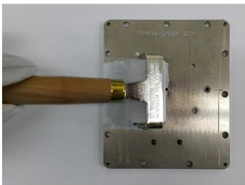
Thermal grease is applied on the heat sink evenly using the rubber roller. Firstly, thermal grease can be distributed in parallel direction with rolling repeatedly.
