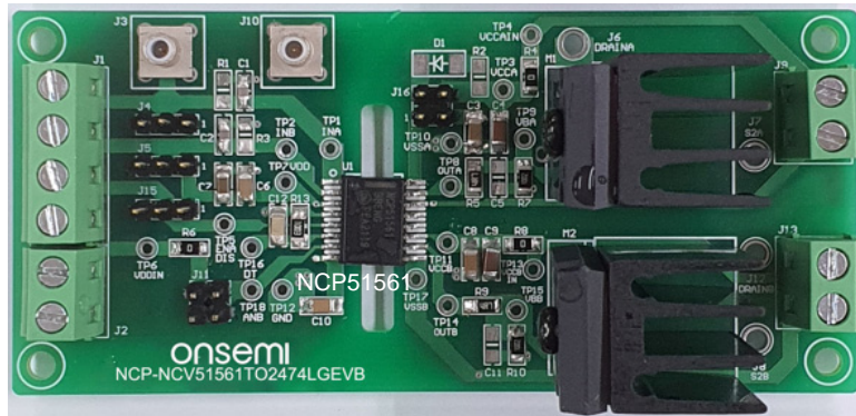
Figure 23. Evaluation Board Picture of Type-B (Top View)
