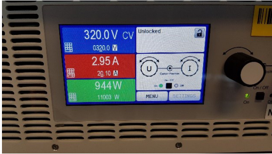
Figure 26. Load Conditions for Current Control Mode. Beginning of the Mode (Above) and End of the Mode (Below)
