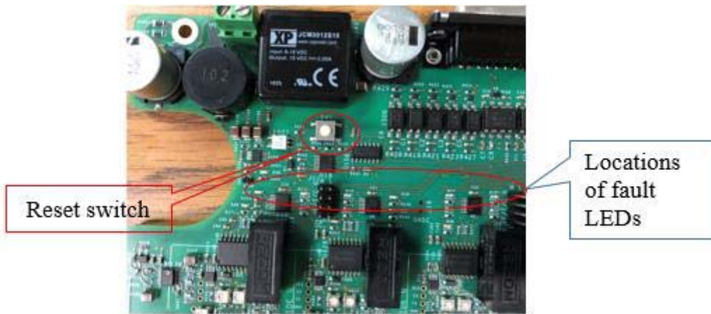
Figure 11. Location of Reset Switch
