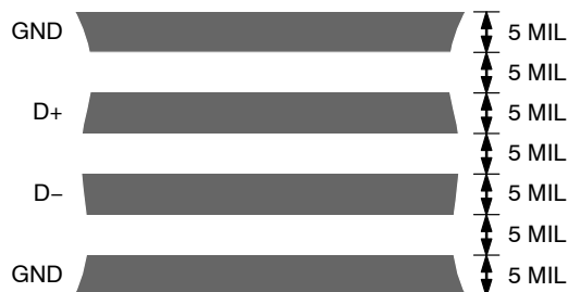
Figure 28. Arrangement of Signal Tracks
