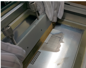
Figure 33. Example (APM19 Package) of Thermal Paste Application Using a Manual Screen Print
