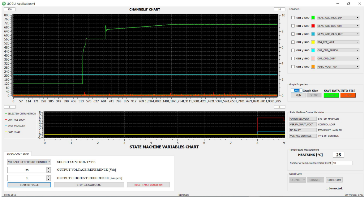
Figure 20. GUI front panel. Bus Voltage
